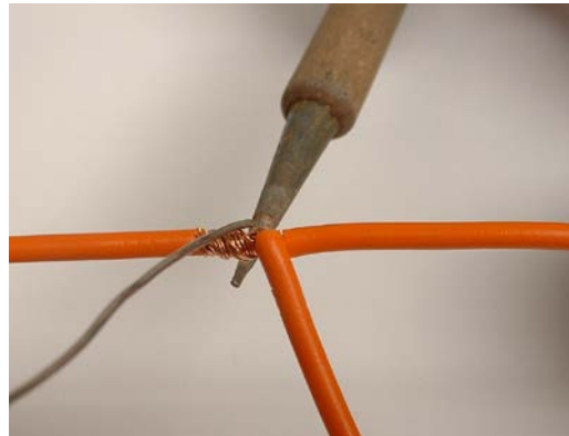
Apply heat to the bottom of the connection and then apply solder slowly as it flows into the wire.
