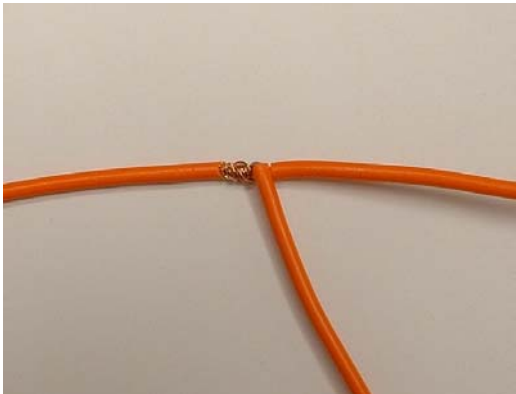
Twist the tap wire into the main wire
