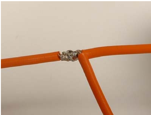
Twist the tap wire into the main wire
