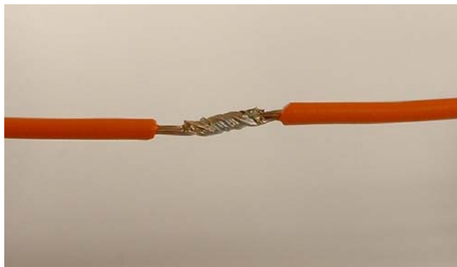
Tightly twist the two wire neatly together
